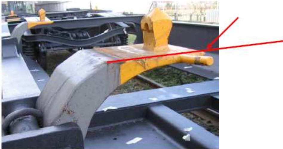
Figure 5 - Horizontal reference plane (limit value 3 mm downwards, with the wagon empty)
